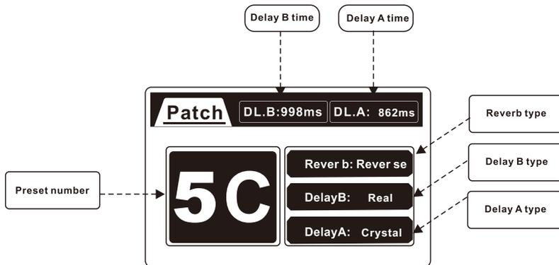
Press the menu button whilst in patch mode on the preset selection screen to enter the Patch Control page.
