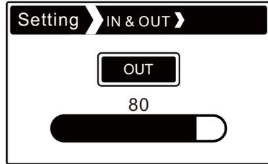
Press the Menu control to change between Input level and Output level
